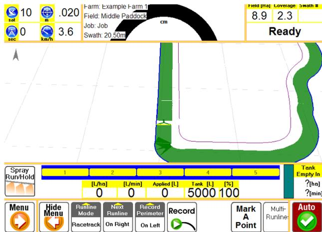
The operator can then complete the coverage for the first lap and, if appropriate, steer toward the Racetrack Runline and engage autosteer.
