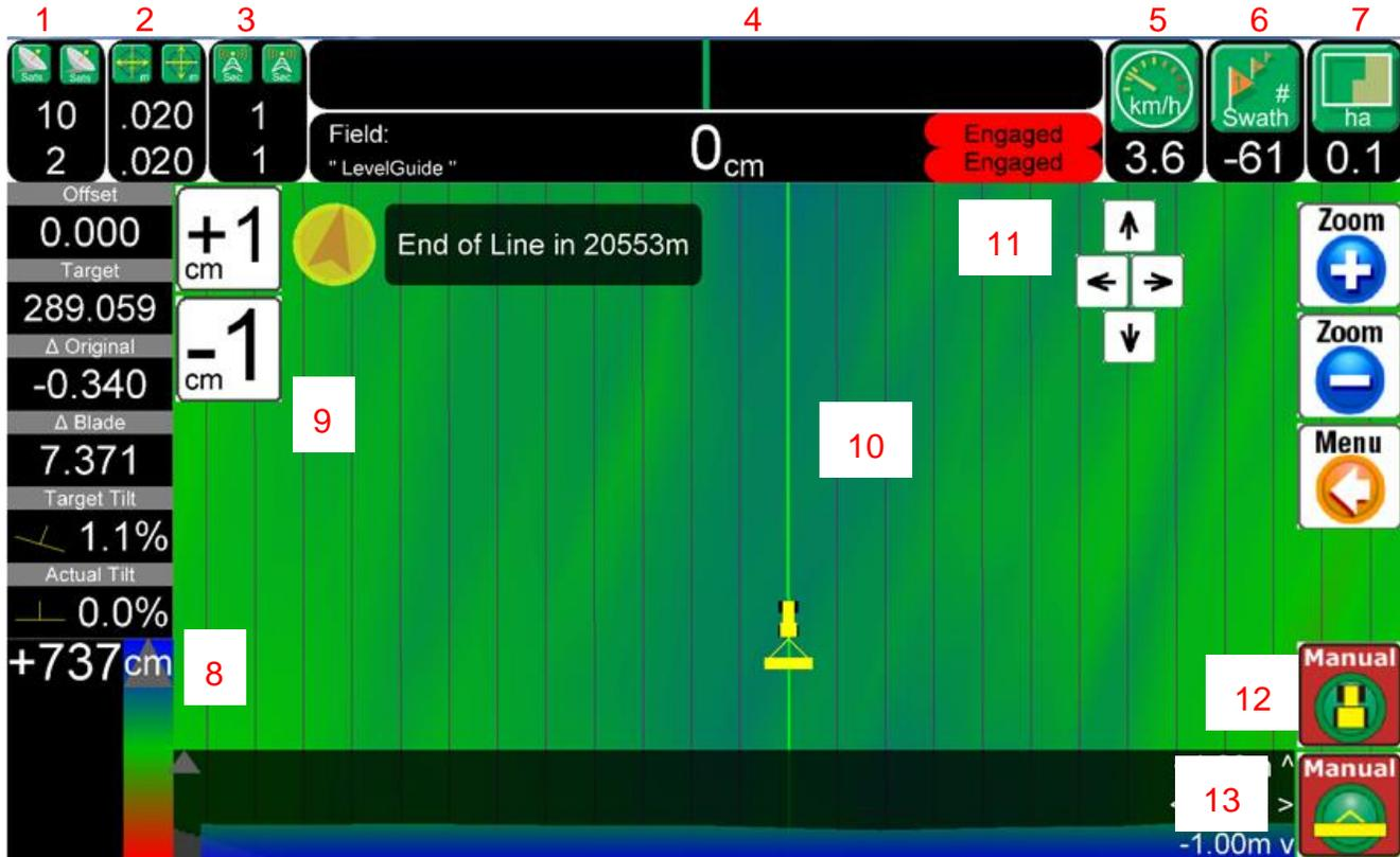
1. Available GPS and Glonass Satellites. Top line is the vehicle GPS Receiver, bottom line is Implement GPS Receiver.
