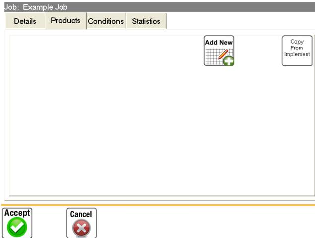
If you have setup the implement previously (best practise) you can copy the relevant properties from the implement, eg number of tanks. In this example the implement was created with one tank and the
