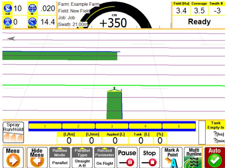
14. The final step is closing the boundary. When AgGuide closes a boundary it does so by drawing a straight line between the current boundary point and the first boundary point. Therefore it is best to start midway down a straight section of fence or at a corner of two straight sections of fence.
